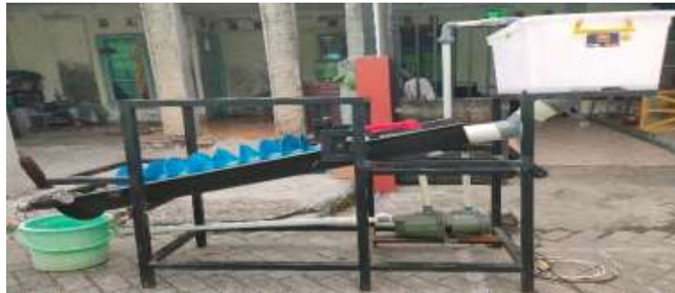
Figure 2. Archimedes' screw turbine
