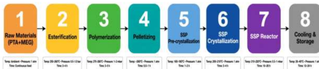
Figure 3.1: Manufacturing Process Flow Chart of PET
