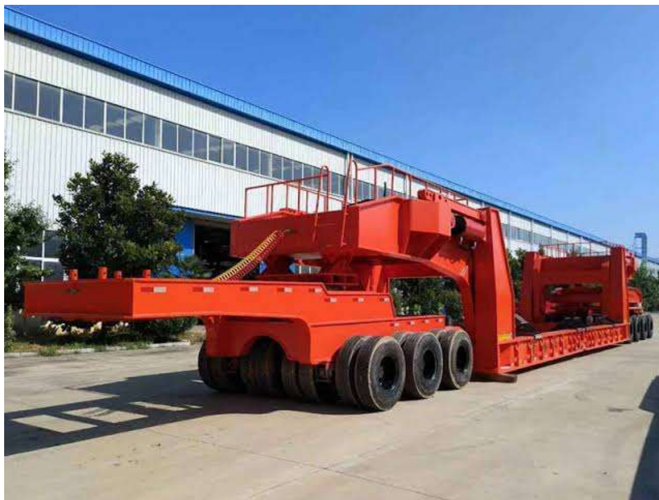
Fig 8: Module Loading (towed hydraulic platform trailers and self-propelled hydraulic platform trailers)
