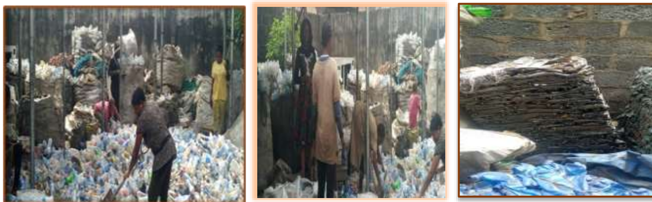
Figure 3a displays the gathering of plastic bottles, Figure 3b demonstrates the segregation process of plastic bottles, and Figure 4a showcases the compacting of plastic bottles into bales before crushing
