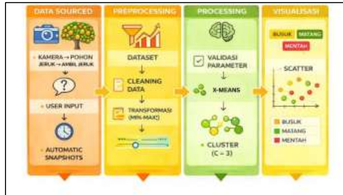
Figure 1. Flowchart of Orange Quality Data Processing in a Real-time Clustering System
